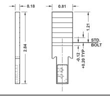
**T37-2**Long bolt can be cut to length required by application
