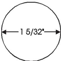
Lock diameter is 1-1/8." Drilled hole should be slightly larger.
