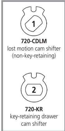
**KEY-RETAINING Function Cam Assembly**
