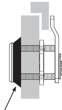
Trim collars pull lock forward allowing it to be used on thinner gauge material thickness.
