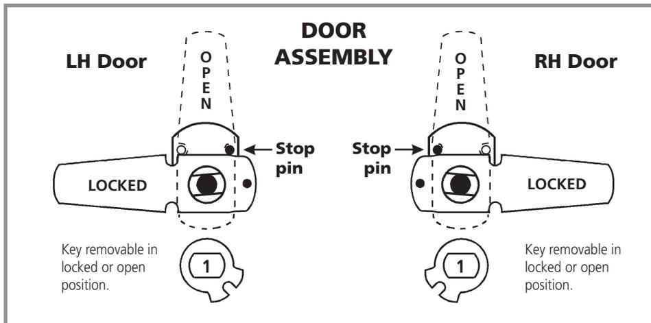
**KEY-RETAINING Function Cam Assembly**
