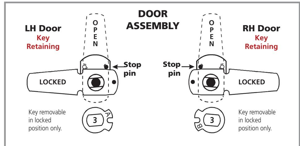
**Assembled with:** 720-3-3 inverted long cam
