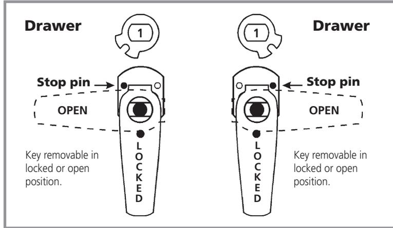
**KEY-RETAINING (direct drive) Function Cam Assembly**
