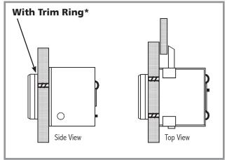
\* Optional trim ring may be required for thin gauge metal doors when used with 7-pin SFIC cylinders
