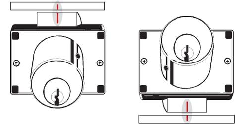
**STRIKE INSTALLATION:** Line up center mark on latch with center mark on strike for correct strike placement.
