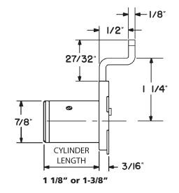
Dimensions with optional long offset bolt installed.
