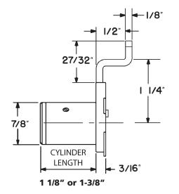
Dimensions with optional long offset bolt installed.
