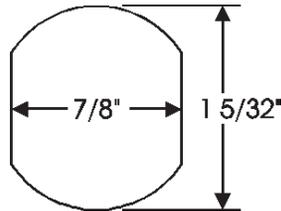
Lock diameter is 1-1/8." Drilled hole should be slightly larger.
