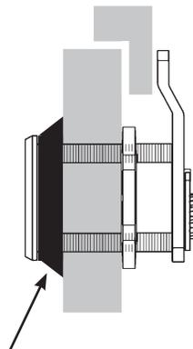
Trim collars pull lock forward allowing it to be used on thinner gauge material thickness.
