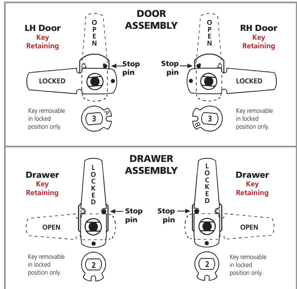
**Assembled with:** 720-3-3 inverted long cam
