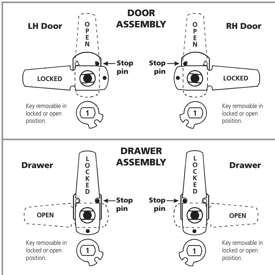
**KEY-RETAINING Function Cam Assembly**
