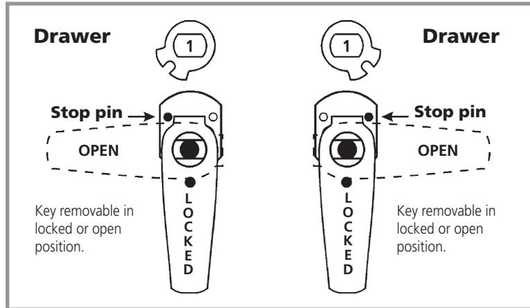
**KEY-RETAINING (direct drive) Function Cam Assembly**
