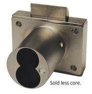
The new **L92V Latch Lock** accepts Schlage full-size interchangeable core cylinders. This lock has a 1-1/8" diameter barrel and will fit up to 1-7/16" material thickness. See also our 777, 888, 920 and 929 series cabinet locks for Schlage full-size IC. Accepts Schlage classic or Primus/Everest or compatible full-size IC.
