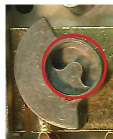
Standard (non-key-retaining) cam disks have a curved slot
