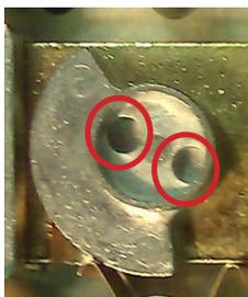
Key-retaining cam disks have two holes
